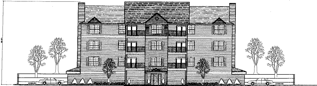
Ⓐ PROPOSED WEST ELEVATION (4:12 ROOF PITCH) SCALE: 1/8" = 1'-0"
