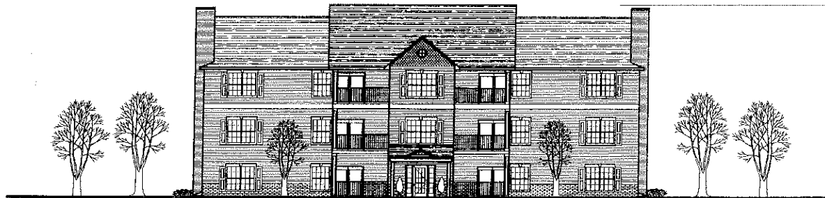
Ⓑ PROPOSED EAST ELEVATION (4:12 ROOF PITCH) SCALE: 1/8" = 1'-0"
